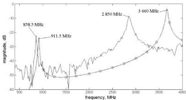
**Figure 3** Simulated and experimental responses of the MTM closed-loop resonator ---o--- simulated ---x--- measured
