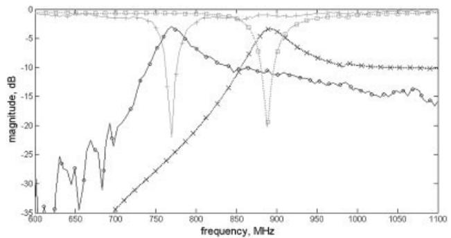
**Figure 5** Simulated and experimental responses of the filter of Figure 2 ---+--- measured  $S_{21}$  ---o--- measured  $S_{41}$  ---□--- simulated  $S_{21}$  ---x--- simulated  $S_{41}$
