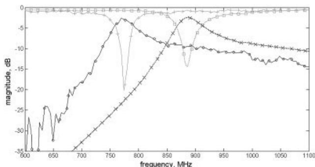
**Figure 4** Simulated and experimental responses of the filter of Figure 1 ---+--- measured  $S_{21}$  ---o--- measured  $S_{41}$  ---□--- simulated  $S_{21}$  ---x--- simulated  $S_{41}$
