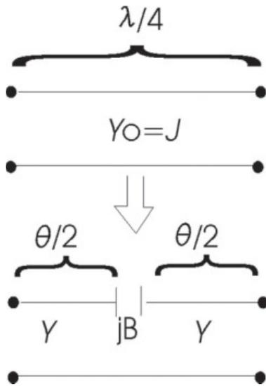
Figure 3 Admittance inverter transformation
