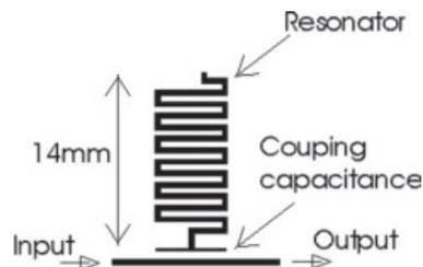
Figure 2 Single meandered resonator coupled to main transmission line
