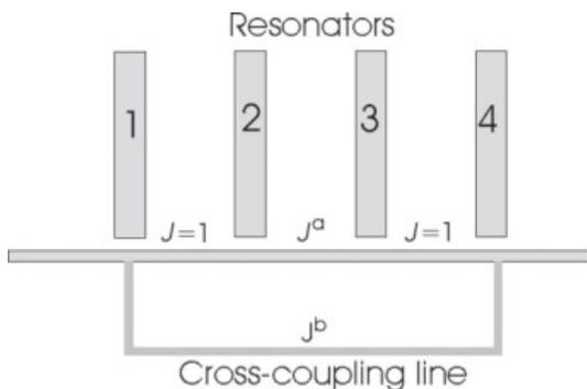
Figure 1 Schematic of quasi-elliptic notch filter
