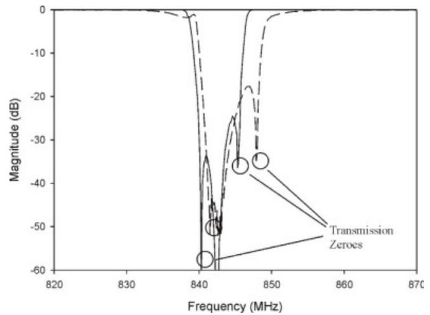
Figure 5 Simulated and measured S21 results of quasi-elliptic notch filter showing the transmission zeroes: — simulated, - - - - measured
