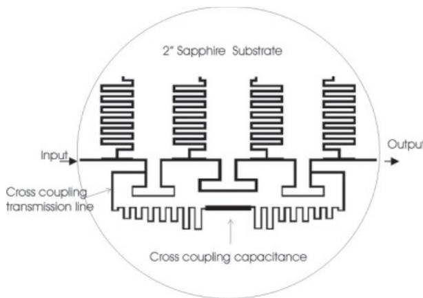
Figure 4 Final layout of the quasi-elliptic filter on 2" sapphire substrate
