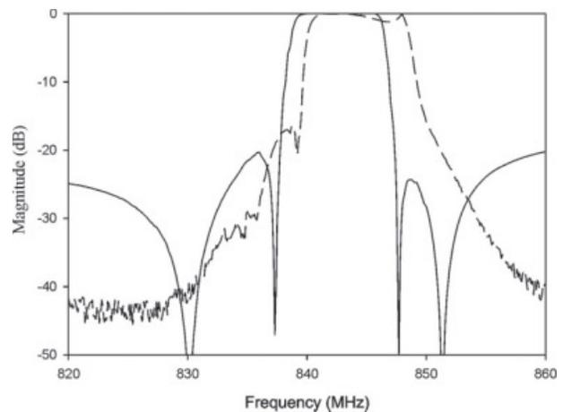
Figure 6 Simulated and measured S11 results of quasi-elliptic notch filter: — simulated, - - - - measured
