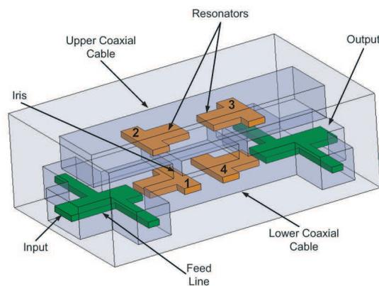
Figure 2: Quasi-elliptic filter topology using vertically adjacent coaxial lines.
