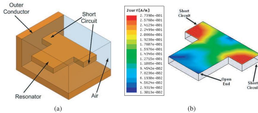
Figure 1: Suspended quarter wavelength resonator. (a) Schematic of the quarter wavelength resonator (side and top walls removed for clarity). (b) Surface current distribution at the resonant frequency of 9.1 GHz.
