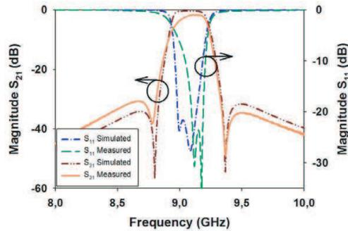
Figure 3: Simulated and measured results for the quasi-elliptic filter implemented on stacked coaxial lines.
