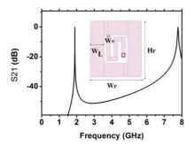
Figure 2. Response of a single uncoupled resonator.
