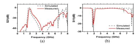
**Figure 4.** Measured and simulated dispersion parameters. (a) Insertion loss and (b) return loss.
