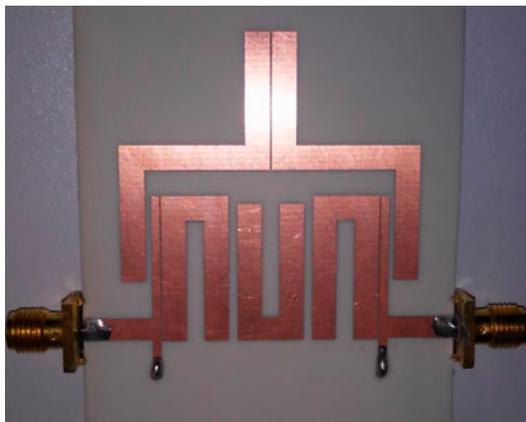
Figure 5. Fabricated filter.
