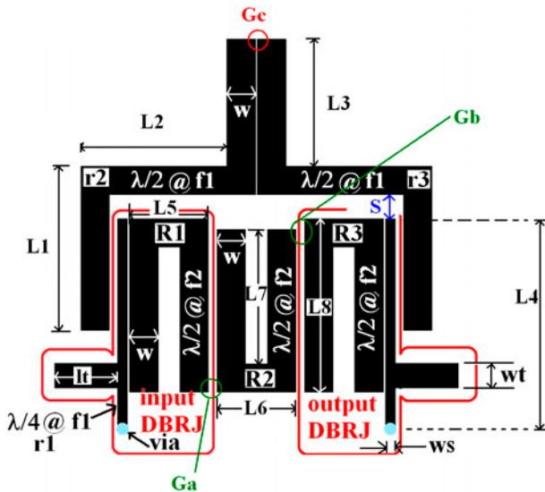
Figure 1. Layout of proposed filter.
