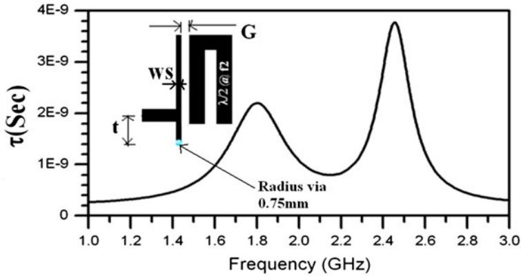
Figure 2.  $S_{11}$  group delay of the resonant junction.
