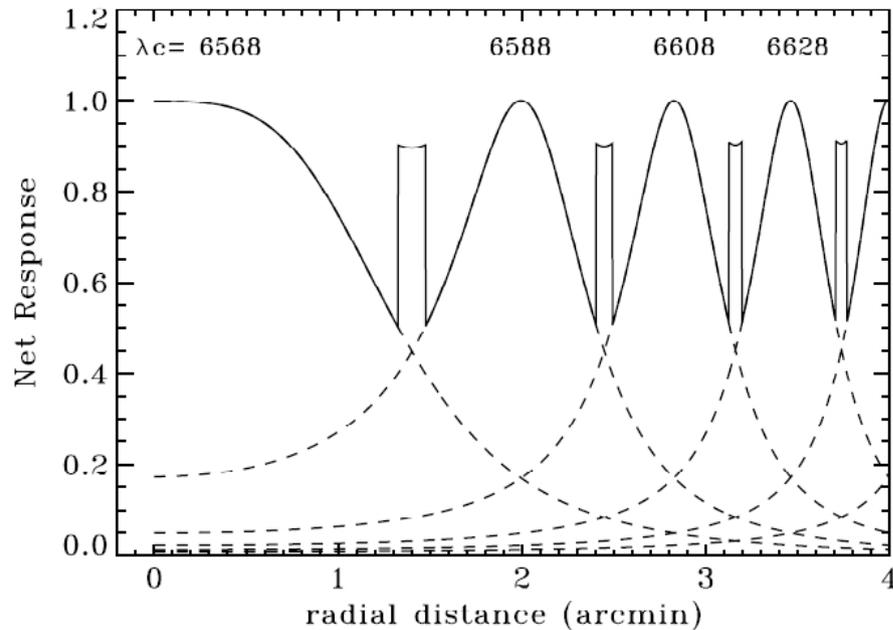
The net response curve for the reconstruction of the H $\alpha$  image. After adding the different image sections, divide the resulting image by the net response.
