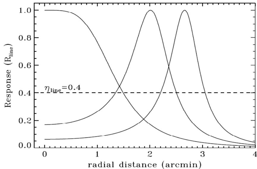
At the reconstruction wavelength, retain only that section of an image where response  $\eta_{\text{line}} > 40\%$ .
